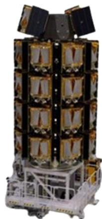
Dispenser holding bunch of satellites thanks to separation nuts
