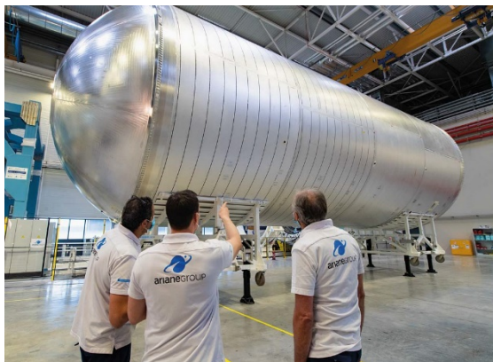
Ariane 6 hydrogen tank at Les Mureaux (France)
