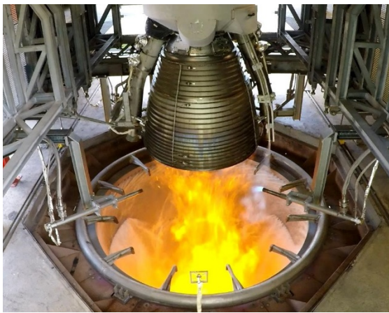
Vulcain 2.1 engine qualification tests on the P5 test stand at the DLR site in Lampoldshausen
