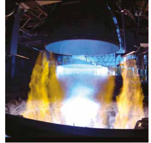
Vulcain 2.1 engine FMI test (Vernon)
