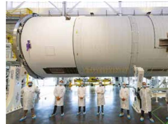
Ariane 6 liquid oxygen tank for combined tests (Les Mureaux)
