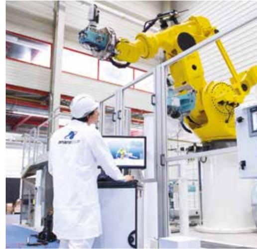
Surface preparation - Laser tracking technology for P120 nozzle (Le Haillan)
